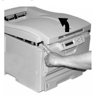
3. Loosen the thumbscrew holding the printer side cover in place.
